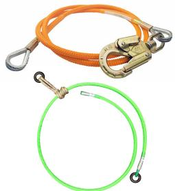
**Flip Lines, Lanyards and Positioning Lanyards:** Flip Lines and Lanyards consist of a variety of precut lengths of rope, typically 8 ft to 15 ft. lengths, that go around the trunk of a tree and are then attached to each side of a climber's saddle on the sewn- in side rings using carabiners and/or snap hooks. Flip lines and Lanyards are adjustable enabling the climber some range of motion while elevated.
